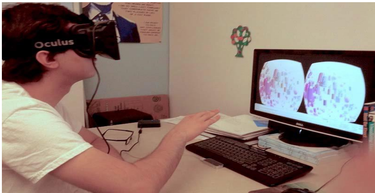
Figure 22 A student using the Oculus Rift™ VR goggles and navigating through the visualized data space using the hand motions and the Leap Motion™ sensor. The computer screen shows the stereoscopic image pair that is being displayed through the VR goggles
